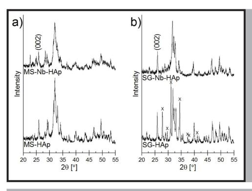
FIG. 3. XRD patterns of powders synthesized through:
