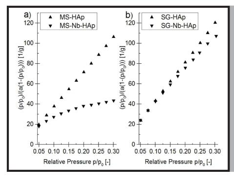
FIG. 2.  $N_2$  adsorption isotherms, used for BET analysis, of powders synthesized through:
